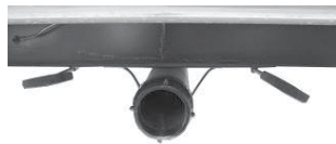
Black/Grey Tank Drain & Valves
