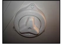
Push knob in to rotate antenna
